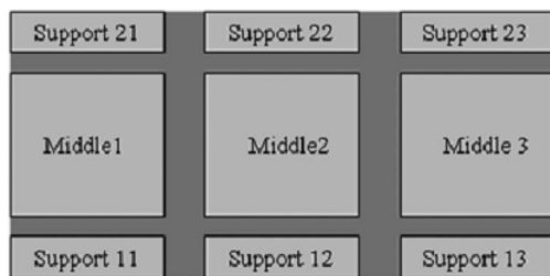
Fig. 7. Notations of the PVDF sensing elements. To generate this pattern, the aluminum coating on one side of a piece of piezoelectric PVDF film was patterned, as shown in this figure.
