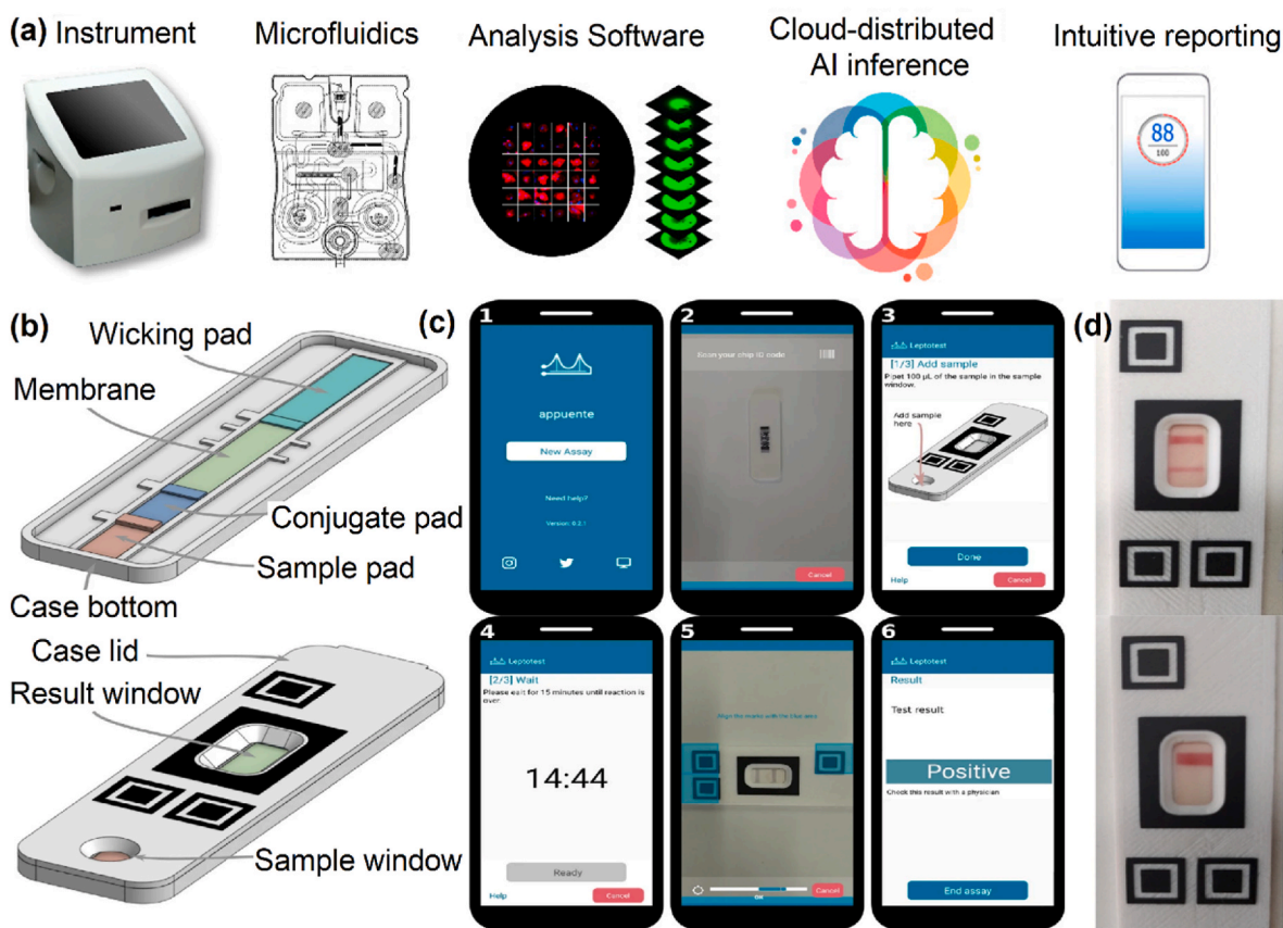
Fig. 7. Integration of IoT and AI with microfluidic devices. (a) Elements of a Smart Diagnostics platform. Adapted with permission from ref. (McRae, Rajsri, Alcorn, & McDevitt, 2022), copyright (2022), MDPI. (b) A 3D render of the LFA parts (top panel) and its cassette (bottom panel). (c) Screenshots of the custom mobile app created using 'appuente', at six running steps: (1) Start new test, (2) scan ID code, (3) add sample, (4) chronometer, (5) automatic imaging and (6) result report. (d) Real examples of LFA chips for positive (top) and negative (bottom) samples. Adapted with permission from ref. (Schaumburg et al., 2022), copyright (2022), Nature.
