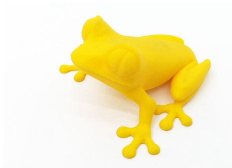
Pict. 26 - the 50-microns treefrog is commonly used as a 3D printing benchmark.
