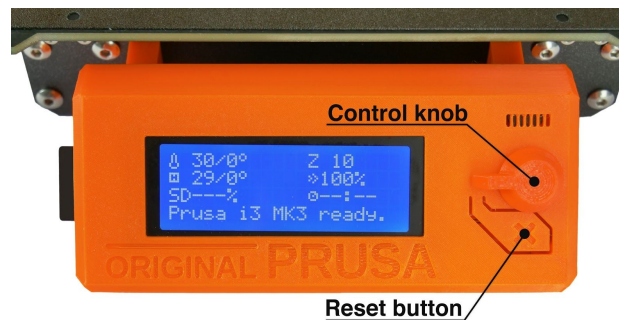
Pict. 15 - LCD screen and control buttons
