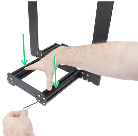
Pict. 46 - Proper way to tighten the frame, plates and aluminum extrusion together.
