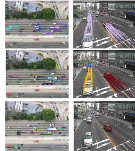
Figure 5: The initial groups from thresholding adjacency matrix (top) and the clustered results for all KLT tracklets (middle) are shown for NYC DOT (right) videos. The final extracted trajectories after spectral clustering and DPGMM are shown in the (bottom) panels.
