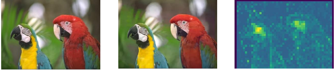
Figure 6.3: Sample decoded image 1 using network trained with clean border Original Image (left), decoded Image (center), lengths of bit-stream for each block (right)
