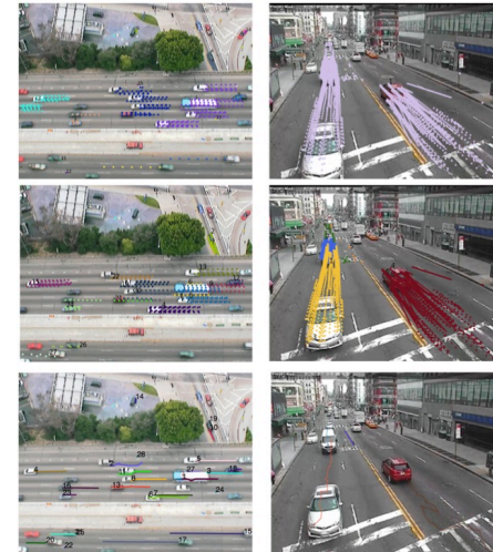
Figure 5: The initial groups from thresholding adjacency matrix (top) and the clustered results for all KLT tracklets (middle) are shown for NGSIM (left) and NYCDOT (right) videos. The final extracted trajectories after spectral clustering and DPGMM are shown in the (bottom) panels.
