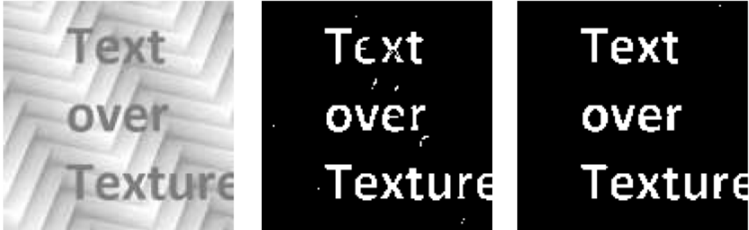
Figure 4.9: The left, middle and right images denote the original image, the foreground maps by using DCT bases for both background and foreground, and using DCT bases for background and Hadamard for foreground respectively.
