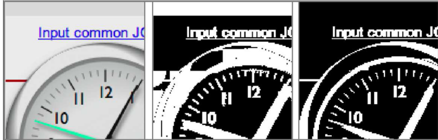
Figure 2.4: Segmentation result for a sample image, middle and right images denote foreground map without and with quad-tree decomposition using the RANSAC as the core algorithm.
