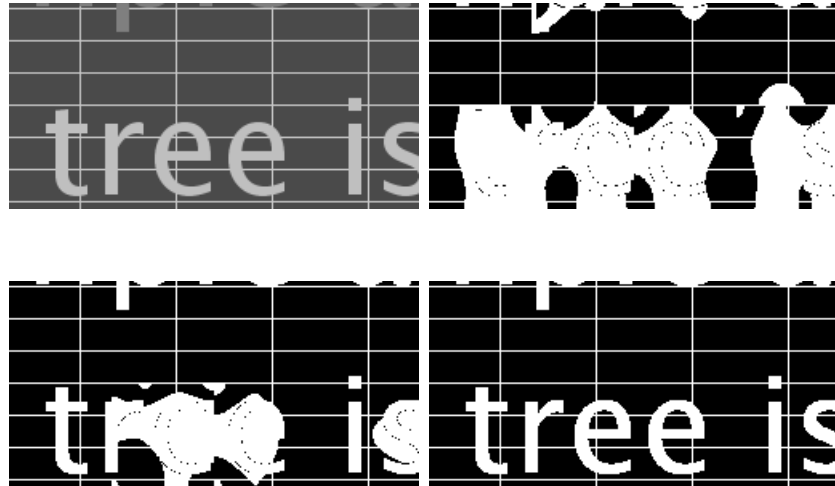
Figure 2.2: The original image (first row), the segmented foreground using least square fitting (second row), least absolute deviation (third row) and sparse decomposition (last row).
