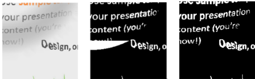
Figure 3.1: The left, middle and right images denote the original image, segmented foreground by hierarchical k-means and the proposed algorithm respectively.
