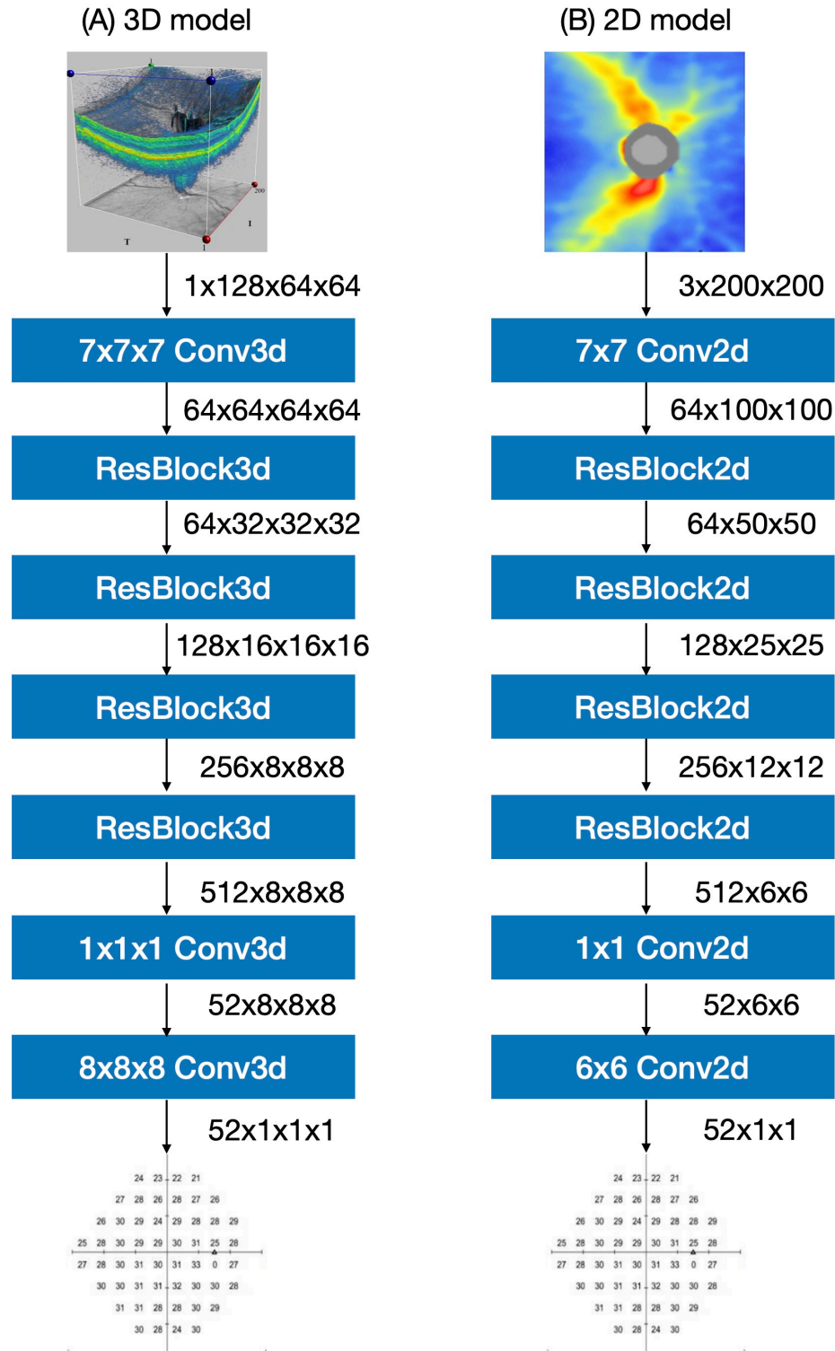
Figure 2.1. Model details. (A): 3D model taking a 3D OCT volume as input ( 1 \times 128 \times 64 \times 64 , channel \times depth \times width \times height ). (B): 2D model taking a 2D RNFL thickness map as input ( 3 \times 200 \times 200 , channel \times width \times height ).
