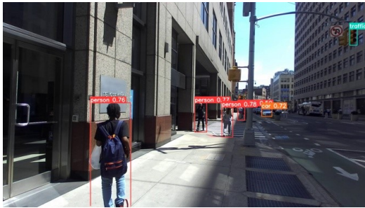
(c) YOLO detection results for (a)
