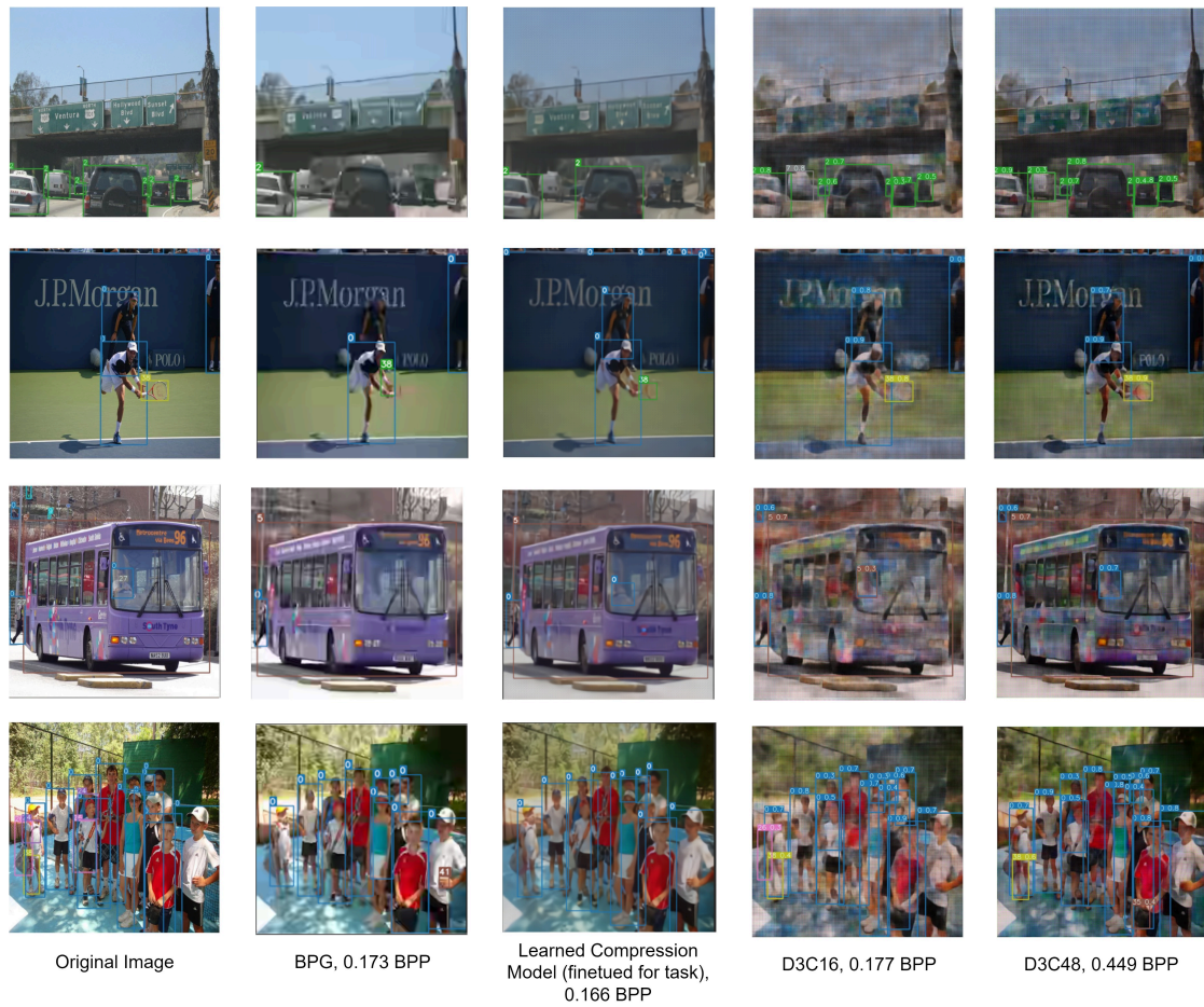
Figure 3.5: Reconstructed images from compressed features from the D3C16 and D3C48 models, compared to decompressed images from BPG and the learned image compression model in [3].
