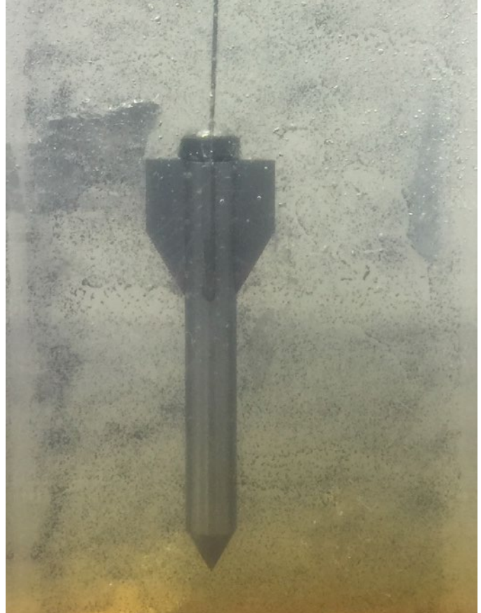
Torpedo anchor after installation in a transparent soil model.
