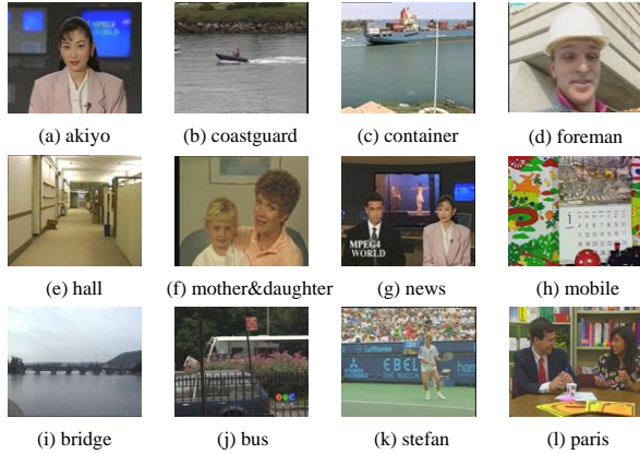
Figure 8: Video pool for generating training and test dataset. All videos are in CIF format and encoded using H.264 by setting Frames Per Second (FPS) and Group of Picture (GoP) size equal to 30.
