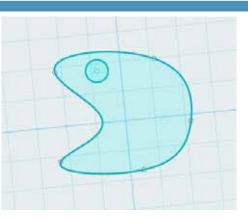
2D to 3D (Extruding) When you take a surface and extrude in a direction, it will continue the surface and give it an edge based on the shape
