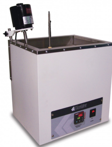
Figure 4: Test Bath Unit for ASTM D130.
