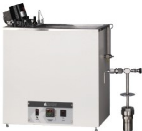
Figure 5: Test Bath Unit and Pressure Vessel for ASTM D525.
