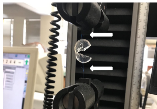
Figure 2: The above image shows a sutured gel being tested using the Instron 5542. The white arrows point to the sutures attached to each end of the gel which are held by the clamps. As the Instron pulls on the sutures, the gel begins to break.
